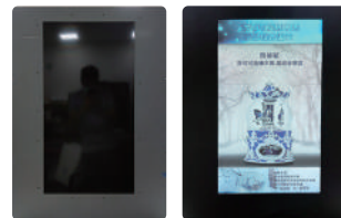
The left picture shows the normal mode, while the right one shows the transparent mode.
